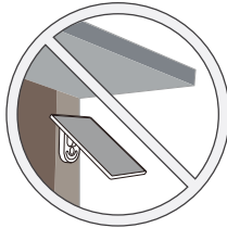
Avoid shade coverage from building eaves
