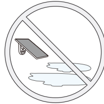
Do not install in water-prone areas
