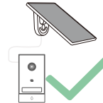
Ensuring the power cable lies naturally without tension
